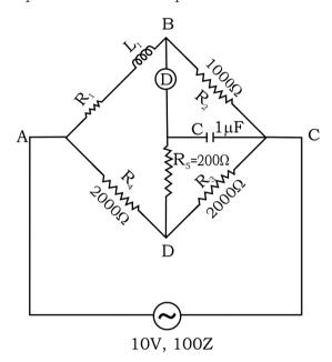
Find  $R_1$  and  $L_1$ , if balance is obtained when  $R_3=R_4=2000\,\Omega$ ,  $R_2=1000\,\Omega$  and  $R_5=200\,\Omega$ ,  $C=1\,\mu\mathrm{F}$ .
